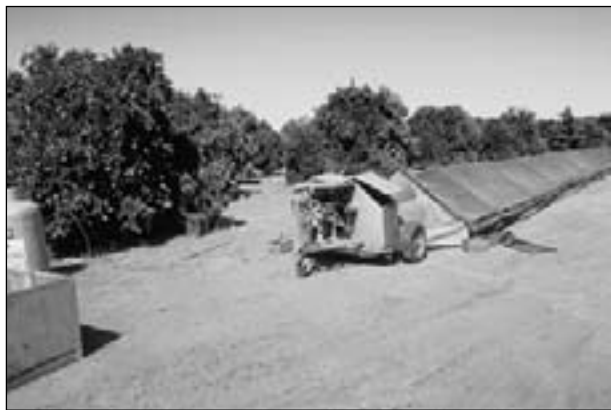
Figure 28.6 A covered "bin dehydrator" with heater unit during operation in Australia. Photo: L. Peter Christensen.
