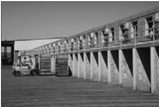
Figure 29.1 Multiple-tunnel raisin dehydrator built of concrete block. Photo: Jack Kelly Clark.
