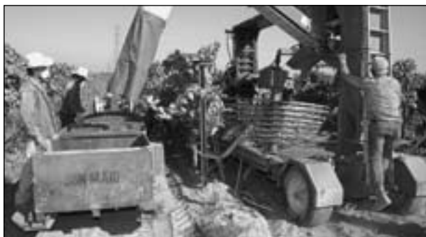
Figure 33.20 A tractor-pulled force-balanced shaker head harvester picking a south-side DOV system. Photo: Jack Kelly Clark.
