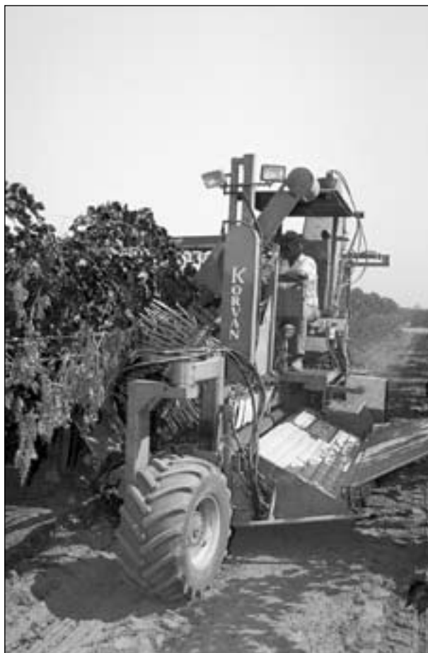
Figure 33.21 A self-propelled lateral shaking (vertirotor head) harvester working in a south-side system. Photo: Jack Kelly Clark.
