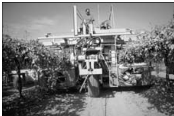
Figure 33.12 The Hiyama harvester picks two half-rows when traveling down each row middle. Photo: L. Peter Christensen.
