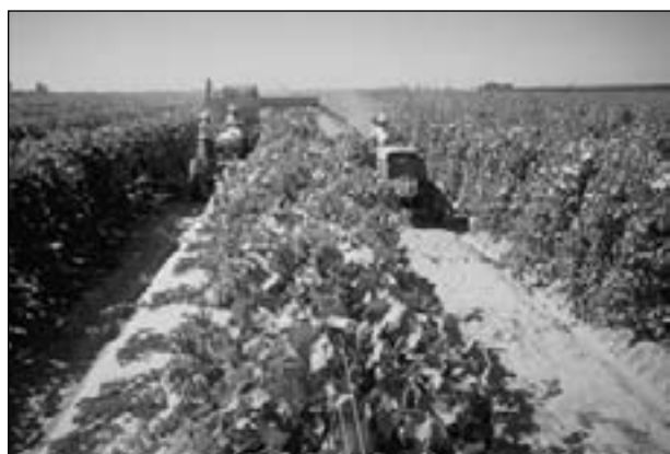
Figure 33.6 Tractor-pulled four-person continuous-tray pickup machine. Photo: L. Peter Christensen.
