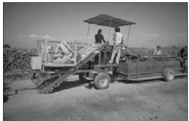
Figure 33.2 A modern raisin roll pickup machine with bin trailer. Photo: L. Peter Christensen.
