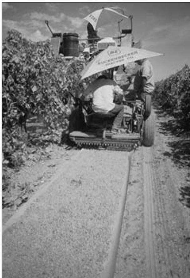
Figure 33.7 Continuous-tray harvest with commercial over-row harvester and spreading machine. Photo: L. Peter Christensen.
