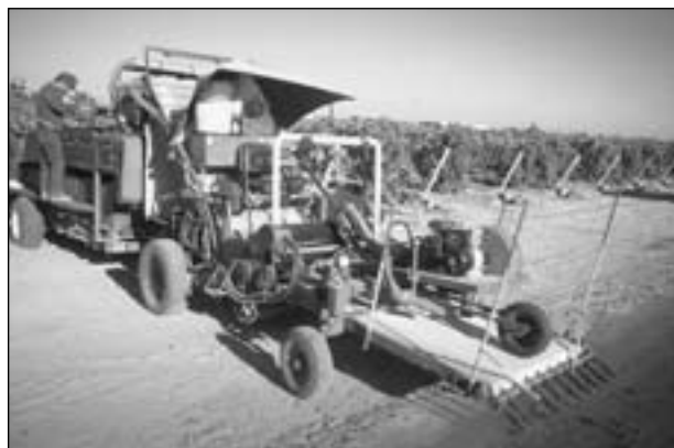
Figure 33.10 Rocca Ranches pickup machine and bin trailer assembly. Photo: L. Peter Christensen.
