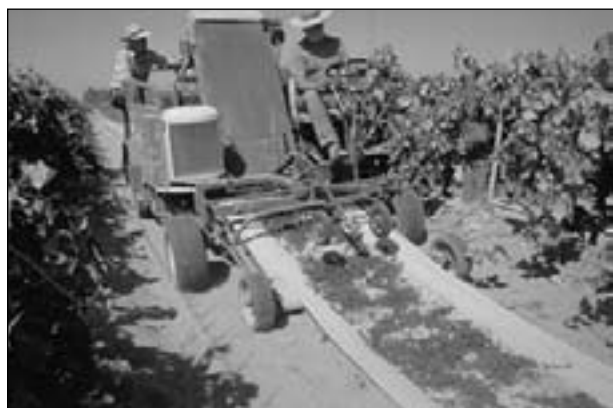
Figure 33.5 Self-propelled two-person continuous-tray pickup machine. Photo: L. Peter Christensen.
