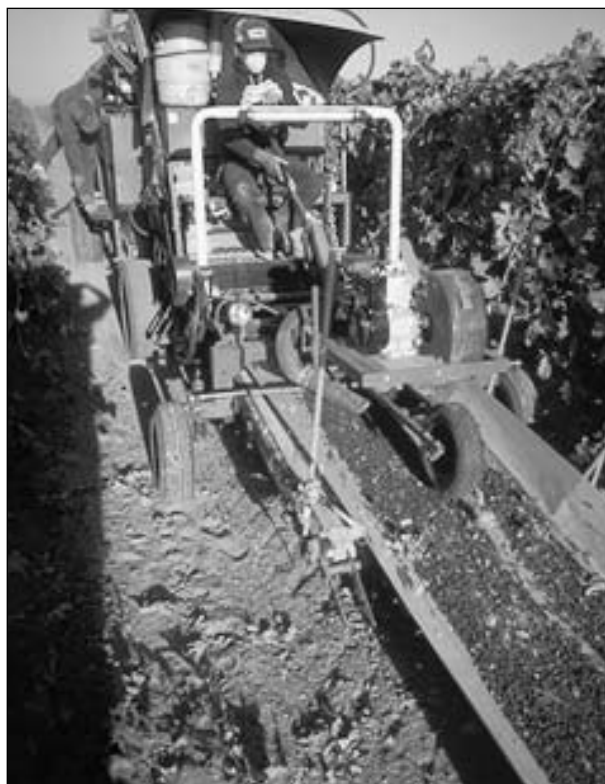
Figure 33.9 Pickup of machine-harvested raisins from a continuous tray 8 days after harvest. Photo: L. Peter Christensen.
