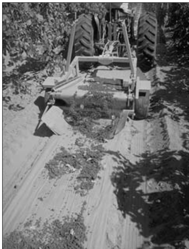
Figure 33.4 Mechanical turning of raisins on a continuous paper tray. Photo: L. Peter Christensen.
