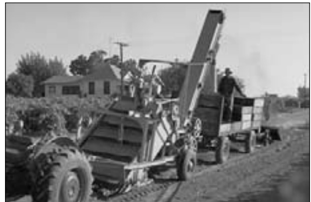
Figure 33.1 An early raisin roll pickup machine invented by Mr. Forbes, a raisin grower near Fowler, California (photo taken in 1968). Photo: L. Peter Christensen.
