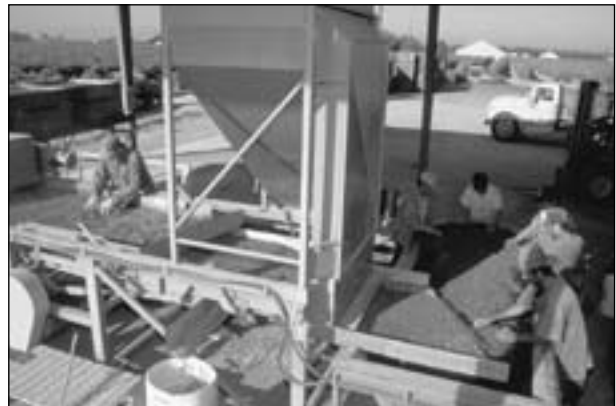
Figure 26.13 A raisin shaker that includes a vacuum attachment on the discharge end to remove light, off-grade raisins. Photo: Jack Kelly Clark.
