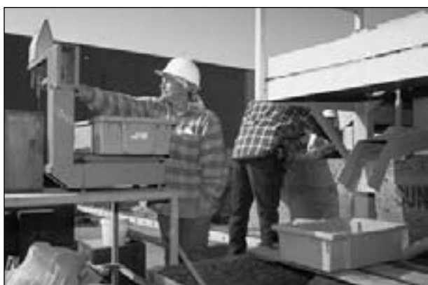
Figure 31.3 Sand that falls through the shaker is collected when bins are dumped. The sand is weighed and the average per bin is deducted from gross weight delivered. Photo: Jack Kelly Clark.
