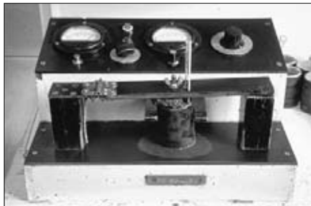
Figure 31.9 Accurate determination of moisture percentage requires that correction be made to compensate for temperature. The thermometer must be placed carefully into the raisin paste; it should not touch the probe or the cylinder. Photo: Jack Kelly Clark.
