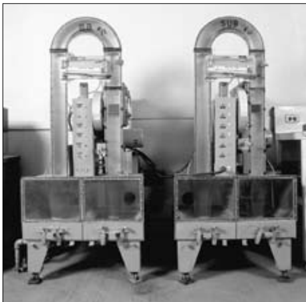
Figure 31.10 Airstream sorter machines are used to determine maturity. “Substandard” (Sstd) or “B or better” (B&B) raisin grades are sorted using a continuous airflow at a constant temperature and pressure. Photo: Jack Kelly Clark.
