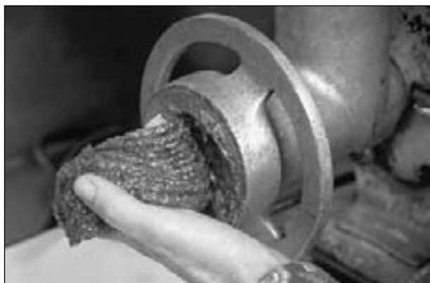
Figure 31.7 Laboratory technicians grind raisins into paste for moisture testing. The paste will be kneaded to remove air and help equalize the moisture in the sample. Photo: Jack Kelly Clark.
